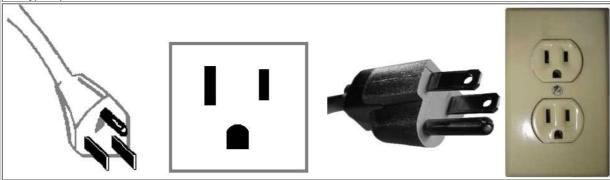
This is a class I plug with two flat parallel prongs and a grounding pin (American standard NEMA 5-15/Canadian standard CS22.2, n°42). It is rated at 15 amps and although this plug is also standard in Japan, it is less frequently used than in North America. Consequently, most appliances sold in Japan use a class II ungrounded plug. As is the case with the type A standard, the Japanese type B plugs and sockets are slightly different from their American counterparts.
