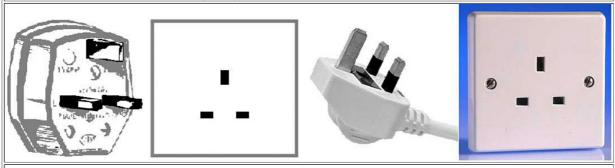
This plug has three rectangular prongs that form a triangle. British Standard BS 1363 requires use of a three-wire grounded and fused plug for all connections to the power mains (including class II, two-wire appliances). British power outlets incorporate shutters on line and neutral contacts to prevent someone from pushing a foreign object into the socket.
