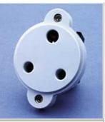
India has standardised on a plug which was originally defined in British Standard 546 (the standard in Great Britain before 1962). This plug has three large round pins in a triangular pattern. It is rated at 5 amps. Type M, which has larger pins and is rated at 15 amps, is used alongside type D for larger appliances in India, Sri Lanka, Nepal and Namibia. Some sockets can take both type M and type D plugs.
